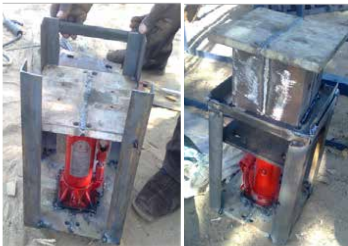
Plate 1. Fabrication process of the briquette making machine
