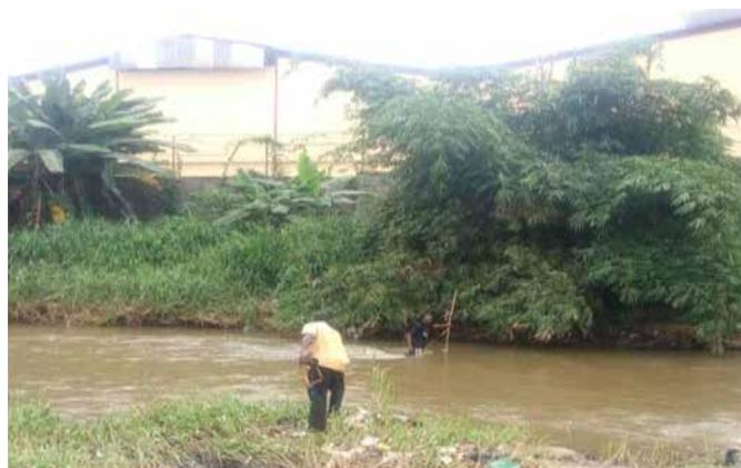
Plate 1: Cross-sectional area determination using measuring tape and bamboo
