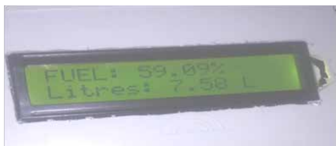
Figure 10: Test result shown when the known value of 7.5 litres of test liquid was measured
