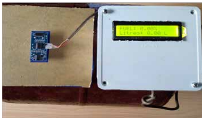
Figure 9: Test result shown when the known value of 0.0 litre of test liquid was measured
