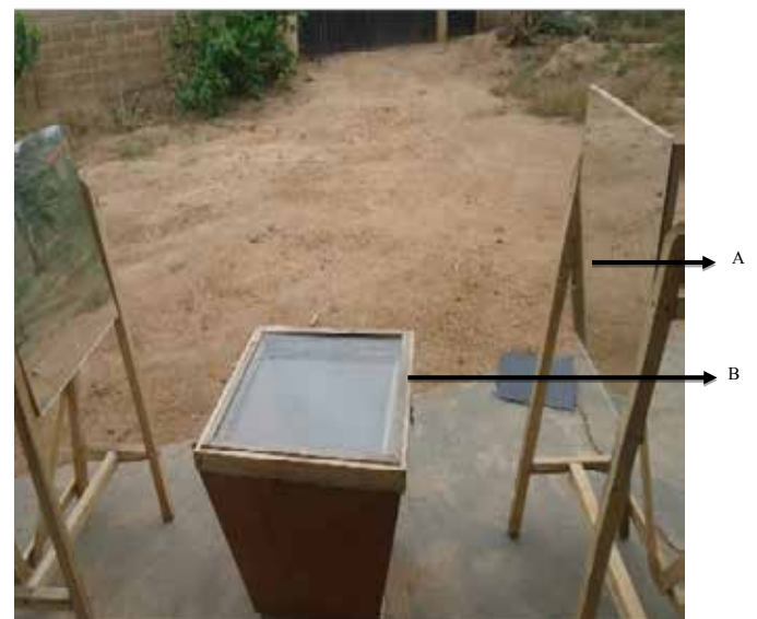
Plate 1: Developed Cooker assembly A is the insolation reflector B is the assembled cooking device.
