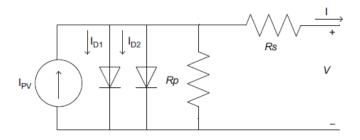
Fig. 4: The equivalent circuit of PV double diode model
