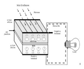
Fig. 1: PV cell (Quaschning, 2005)
