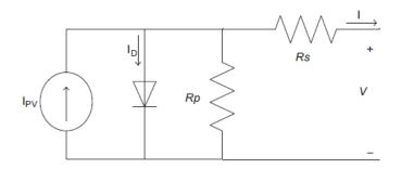
Fig. 3: The equivalent circuit of PV single diode model
