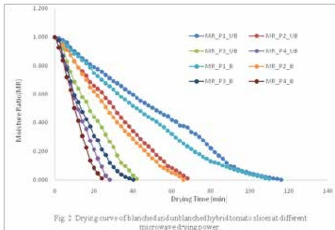
Fig. 2 Drying curve of blanched and unblanched hybrid tomato slices at different microwave drying power.
