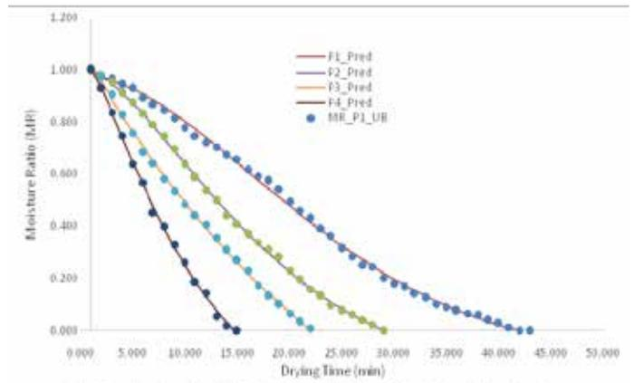
Fig 7. Experimental and predicted Drying Curves of Unblanched Eva-F1 tomato slices at various microwave power using Demir model
