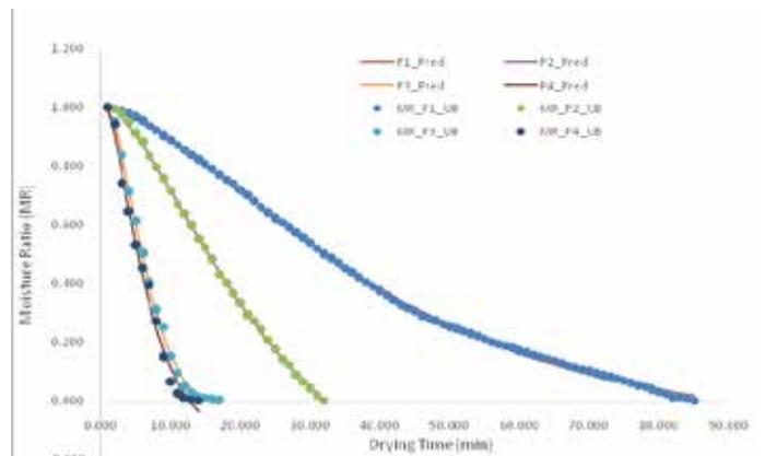
Fig 8. Experimental and predicted Drying Curves of Unblanched yoruba tomato slices at various microwave power using Demir model
