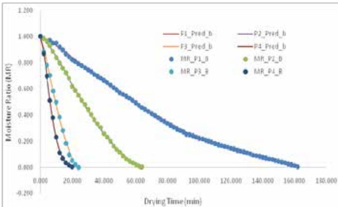
Fig 5. Experimental and predicted Drying Curves of blanched yoruba tomato slices at various microwave power using Demir model
