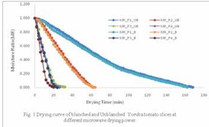
Fig. 1 Drying curve of blanched and Unblanched Yoruba tomato slices at different microwave drying power.
