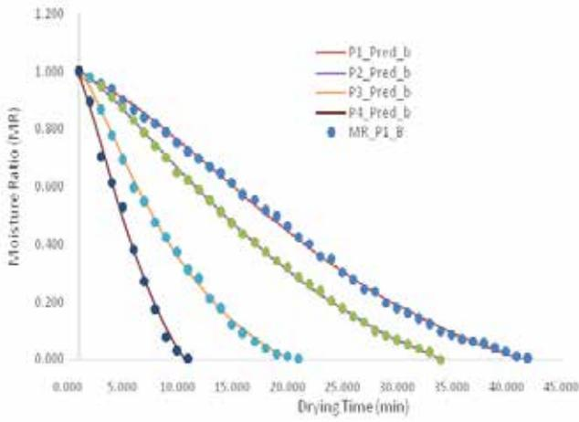
Fig 4. Experimental and predicted Drying Curves of blanched Eva-F1 tomato slices at various microwave power using Demir model
