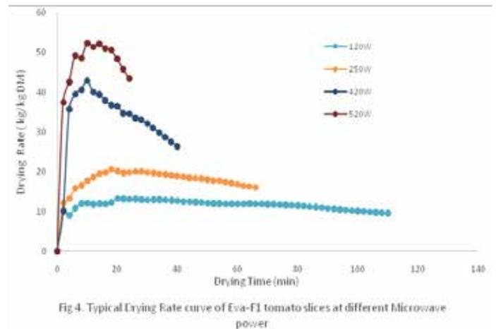
Fig 4. Typical Drying Rate curve of Eva-F1 tomato slices at different Microwave power
