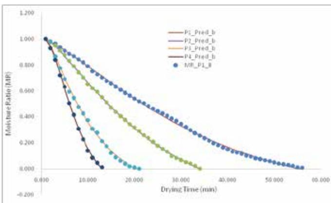
Fig 6. Experimental and predicted Drying Curves of blanched UC-82B tomato slices at various microwave power using Demir model
