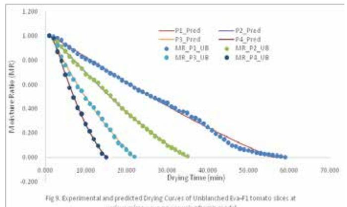
Fig 9. Experimental and predicted Drying Curves of Unblanched Eva-F1 tomato slices at various microwave power using Demir model
