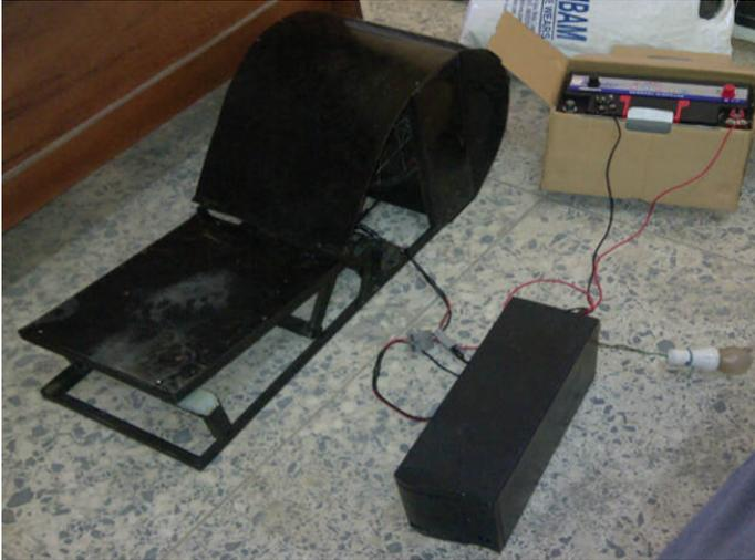
Fig. 7: The footstep unit, inverter, and the battery
