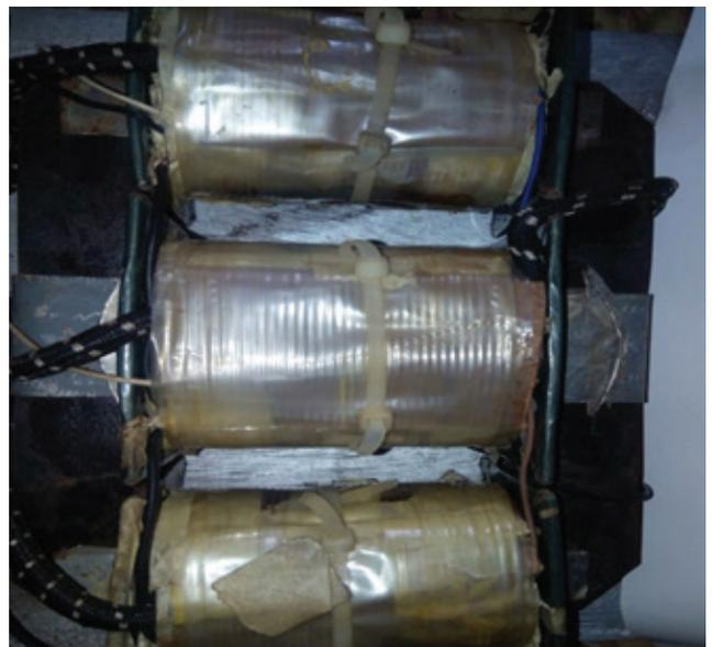
Fig. 4: Three-phase, three-leg, core-type voltage transformer.
