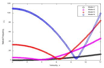
Figure 3: Natural frequency ( $\omega$ 1) profile as a function of mode for the case L = 150 m, h = 100 m,  $\delta$  = 0.2
