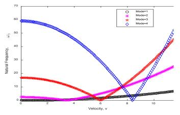
Figure 7: Natural frequency ( $\omega$ 1) profile as a function of delta in the absence of Coriolis effect for the case L = 150 m, h = 100 m,  $\delta$  = 0.2
