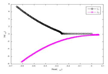
Figure 9: Imaginary natural frequency versus real Natural frequency as a function of poles for the case L = 150 m, h = 100 m, n = 1,  $\delta$  = 0.2
