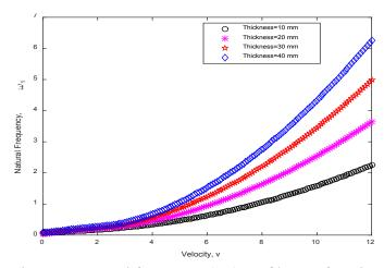
Figure 5: Natural frequency ( $\omega$ 1) profile as a function of pipe thickness for the case L = 150 m, h = 100 m, n = 1
