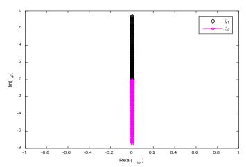
Figure 10: Imaginary natural frequency versus real Natural frequency in the absence of Coriolis as a function of poles for the case
