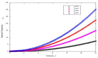
Figure 2: Natural frequency ( $\omega$ 1) profile as a function of delta for the case
