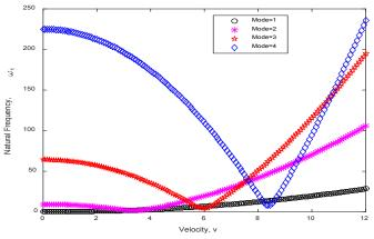
Figure 8: Natural frequency ( $\omega$ 1) profile as a function of mode without seawave effect for the case L = 150 m, h = 100 m,  $\delta$  = 0.2
