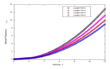
Figure 4: Natural frequency ( $\omega$ 1) profile as a function of L for the case  $\delta = 0.2$ , h = 100 m, n = 1
