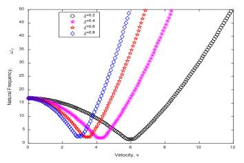
Figure 6: Natural frequency ( $\omega$ 1) profile as a function of delta for the case L = 150 m, h = 100 m, n = 3
