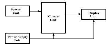
Figure 1: Block diagram of IR-based bidirectional counter
