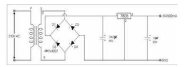
Figure 2: Circuit diagram of power supply unit
