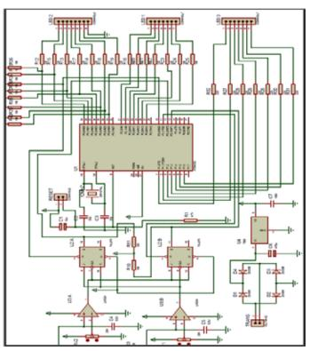
Figure 5: Circuit diagram of IR-based bidirectional counter
