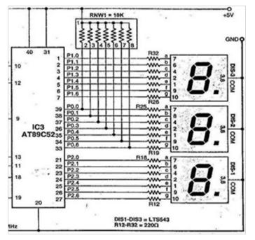
Figure 4: Connection between AT89C52 pins and LTS543 CC display module
