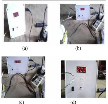
Figure 8: Results of performance tests carried out on the constructed IR-based bidirectional counter (a) power ON, counter displays 000 (b) maximum possible count, counter displays 999 (c) Response after 24 interrupts of INT0, counter displays 024 (d) Response after 21 interrupts of INT1 using (c) as takeoff, counter displays 003
