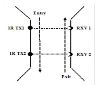
Figure 7: Sensors arrangement at an entrance
