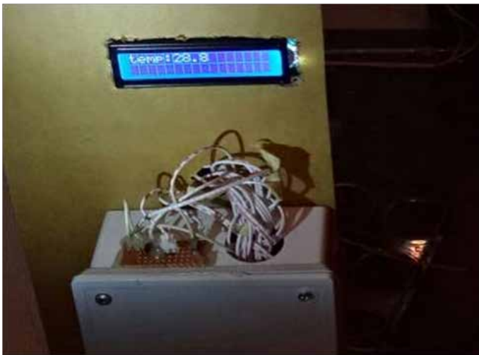
Fig. 5: Plate showing response of the constructed device to change in temperature when the temperature is temperature is 28.8°C (between 25°C and 29°C)
