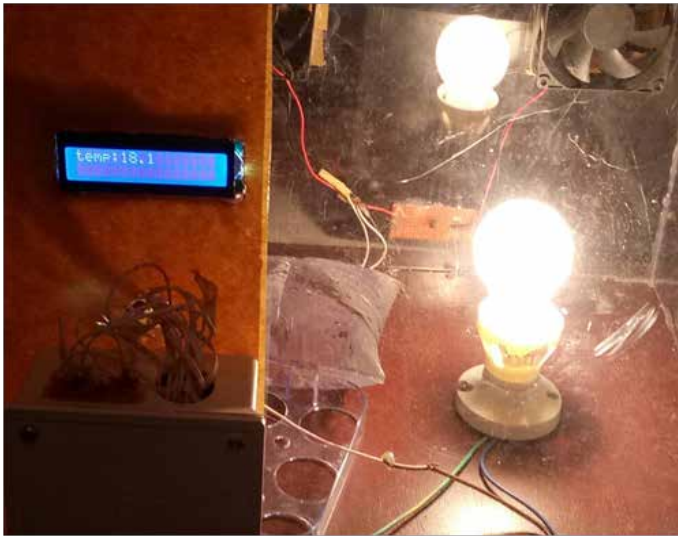
Fig. 5: Plate showing response of the constructed device to change in temperature when the temperature is (a) 18.1°C (below 25°C)
