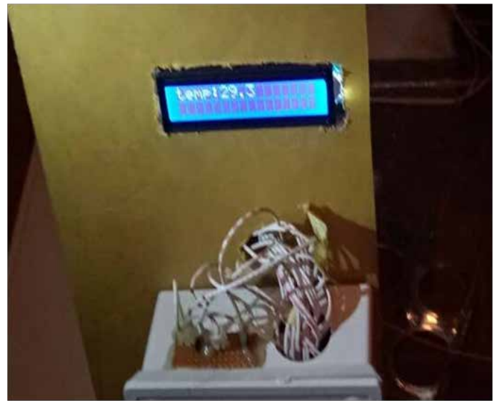
Fig. 7: Plate showing response of the constructed device to change in temperature when the temperature is 29.3°C (above 29°C)
