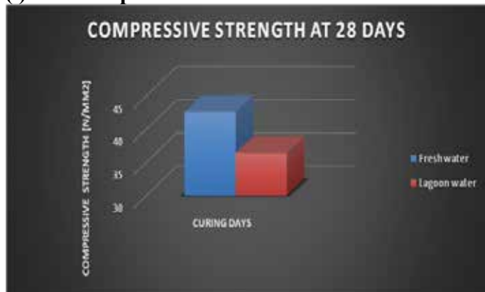
Figure 1: Average Compressive Strength of C-40 Concrete.
