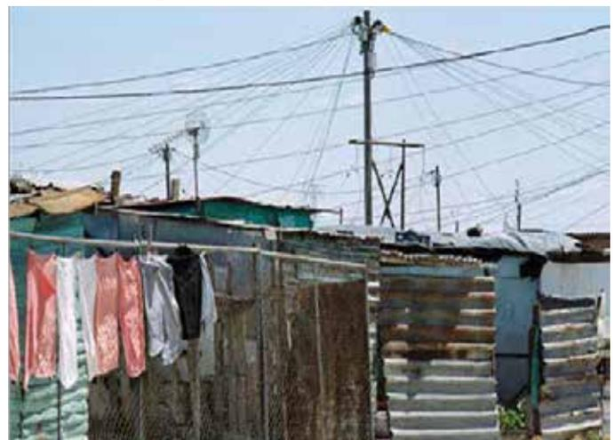
Figure 1: Indiscriminate Connection to an Electricity Supply Pole
